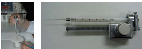
Figure 12: Topical application (A) anaesthetized planthoppers on watchglass wrapped with gauze, (B) Hamilton repeating dispenser and microsyringe.
