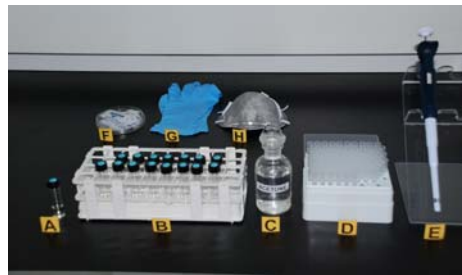
Figure 9: Materials for preparation of serial dilutions (A) stock solution, (B) 6 ml screw cap vials with label, (C) technical grade acetone, (D) pipettor tips, (E) pipettor, (F) parafilm strips, (G) disposable nitrile gloves, (H) disposable mask.
