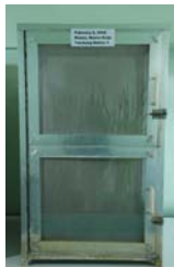
Figure 4: Aluminum rearing / oviposition cage (56.5 cm x 56.5 cm x 91.5 cm) with aluminum wire mesh on 3 sides, top and doors for ventilation.
