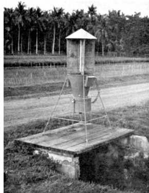
A dry fluorescent light trap
